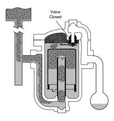
**3.** As the entering condensate starts to fill the bucket, the bucket begins to exert a pull on the lever. As the condensate continues to rise, more force is exerted until there is enough to open the valve against the differential pressure.
