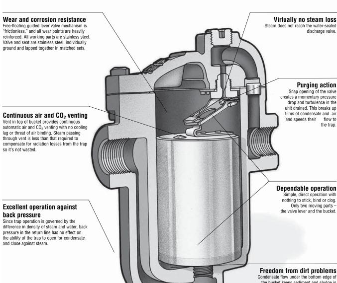
concensate riow under the bottom edge of the bucket keeps sediment and sludge in suspension until it is discharged with the condensate. Valve orifice opens wide and closes tightly. No buildup of dirt or close clearances to be affected by scale.
