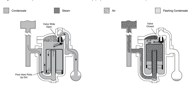
2. Steam also enters trap under bottom of bucket, where it rises and collects at top, imparting buoyancy. Bucket then rises and lifts valve toward its seat until valve is snapped tightly shut. Air and carbon dioxide continually pass through bucket vent and collect at top of trap. Any steam passing through vent is condensed by radiation from trap.
